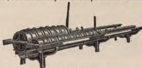
Fig. 219. Steel combination cheese-press.
